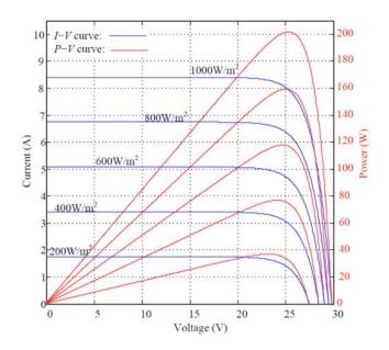
Temperature Coefficient of Isc: 0.0686%/℃ Temperature Coefficient of Voc:- 0.362%/℃ Power Temperature Coefficient:- 0.4359%/℃ NOCT:43.6±1℃
