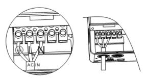
③ Properly connect the AC output wire according to the wire sequence and terminal position shown in the figure below. Please connect the ground wire first, and then the live wire and the neutral wire. The ground wire is connected to the grounding screw hole on the cabinet through the O-type terminal.
