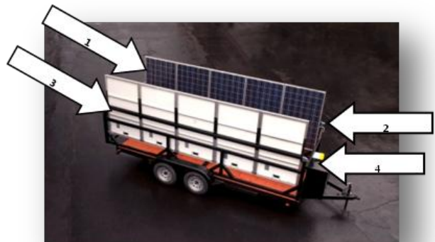
Figure 3 The four locations of the spring-loaded, locking pins
