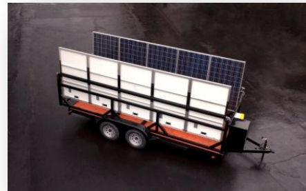
Figure 1 Vertical position of the PV panels for transporting.
