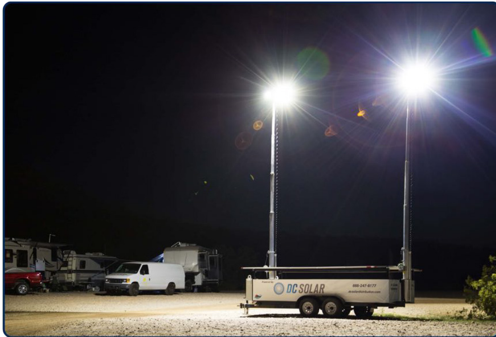
Figure 25 Light Towers in Use
