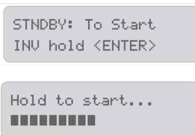
Figure 1 Startup Inverter Display
